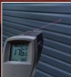
Heat gun pointed at Abtco vinyl siding at a temperature of 176.5 F. No distortion from the intense heat
